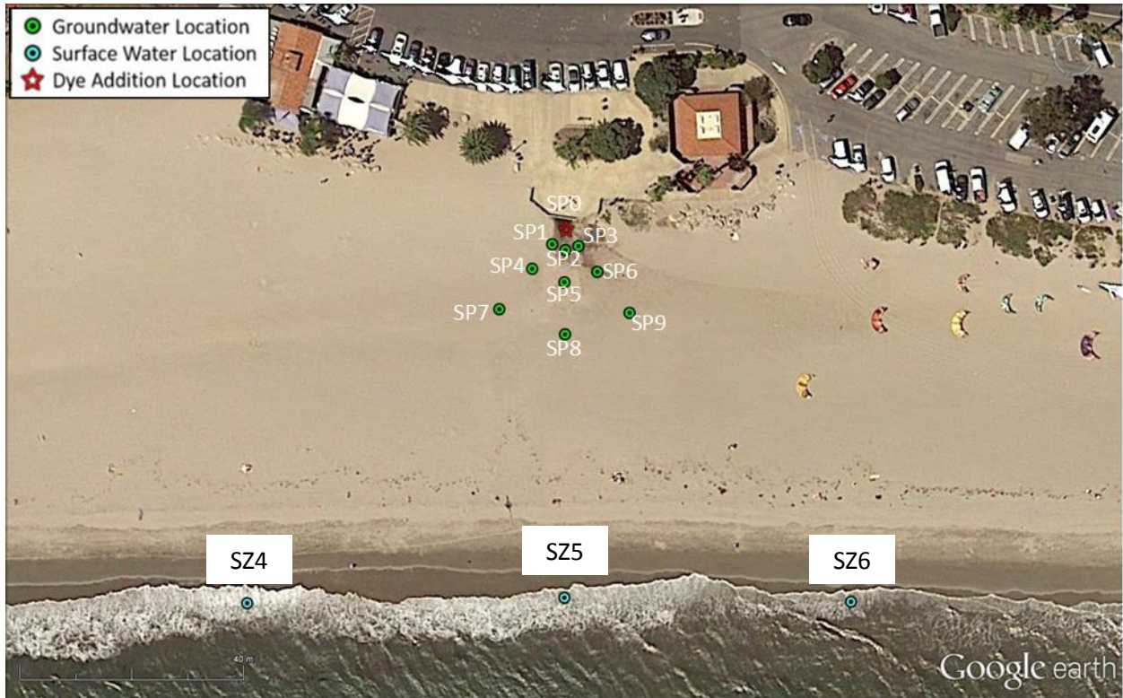
Fig. S12 Groundwater (SP1-SP9) and surface water (SZ4-SZ6) sampling locations at the Honda Creek culvert outlet, LB. SP0 was installed to introduce dye to the subsurface.
