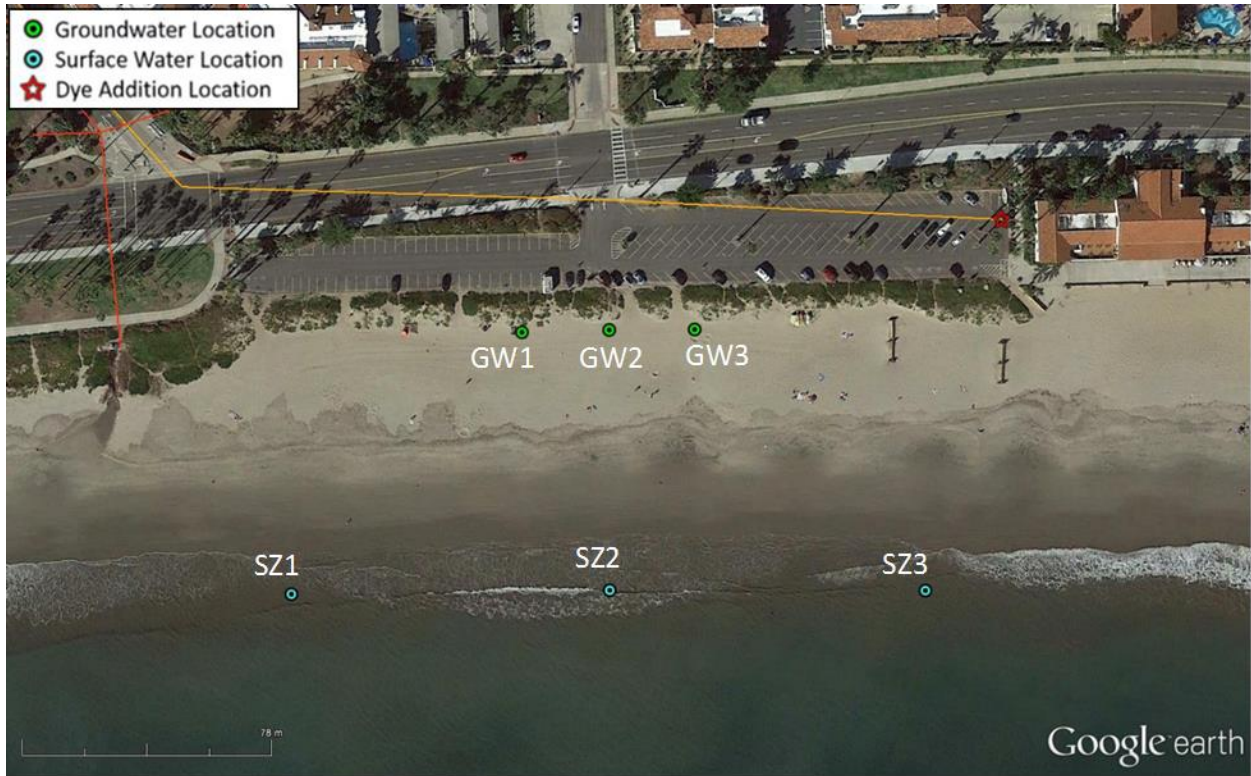
Fig. S15 Groundwater (GW1-GW3) and surface water (SZ1-SZ3) sampling locations at EB for assessing sanitary sewer leakage beneath the parking lot west of the Cabrillo Bathhouse in 2016.
