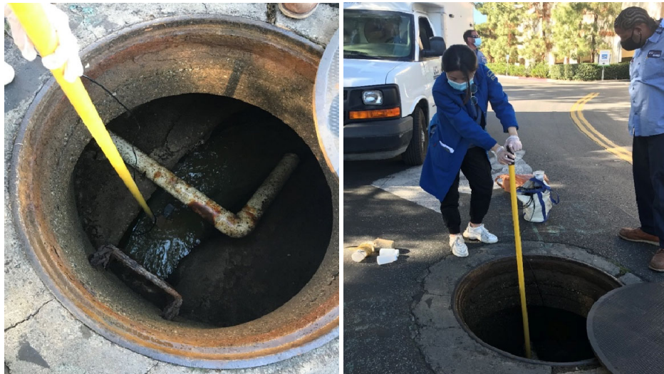
Figure 3-6. Pictures of a Sampling Event When Flowrate Was Measured at the UCI-MH-A Site.
